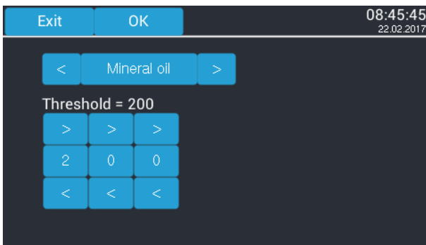
Fig. 14 – Display, selection of insulating liquid and parameterization of H 2 limit value
